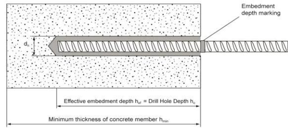
**Table A2: Installation details for rebar**
